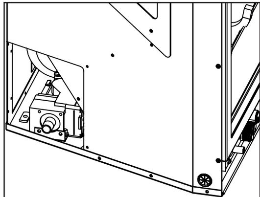
Figure 26:  $\frac{3}{8}$ " NPT Male Pipe Nipple with Cover Removed.
