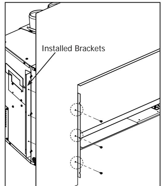
**Figure 35: Screw Installation Locations.**
