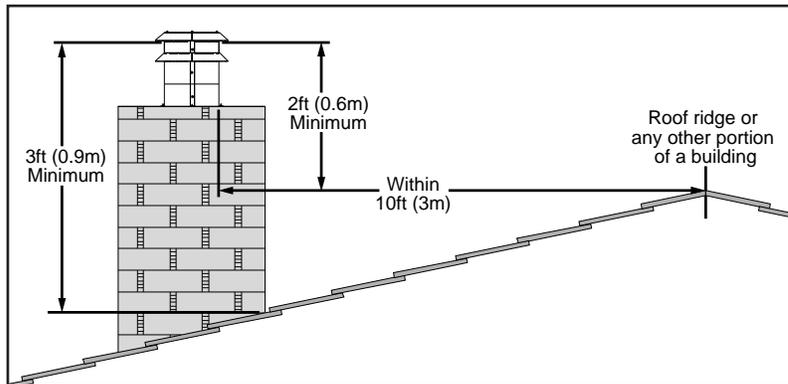
**Figure 20: Roof Clearances.**
