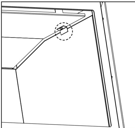
**Figure 40:** Remove the clips which secure the side panels and then pull the bottom of the panels towards the center of the firebox.
